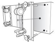
\* BUP300S mounting brackets (sold separately) can be used for easy mounting on an EIA/JIS 19-inch rack. Refer to the BUP300S instruction manual for more details.
